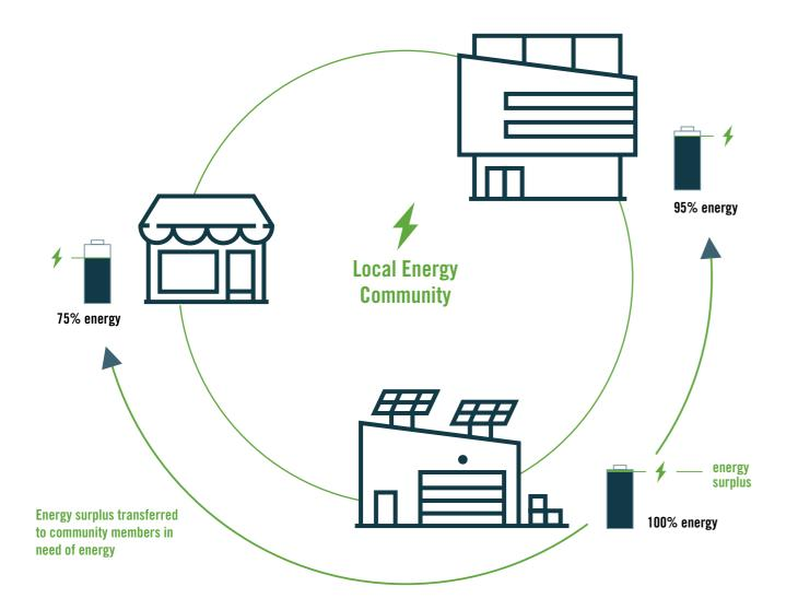
Although, according to the applicable legislation, a surplus of production can only be placed on the power grid without it being possible to share the energy with the local community, this project is investigating a low regulation zone in which electricity produced can be purchased by different parties in the vicinity, which reduces dependence on the public power grid.
